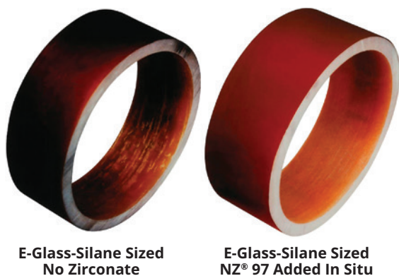
FIGURE 4 » The control on the left shows the E-glass (silane sized) fiberglass windings projecting through the anhydride-cured epoxy wall, while the Ken-React® NZ® 97-containing sample on the right, having the same type and degree of fiberglass reinforcement, shows no apparent fiberglass presence due to the almost complete interfacial adhesion of the epoxy to the fiberglass. Copyright Kenrich Petrochemicals, Inc.
