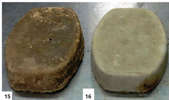
FIGURE 3 » The use of titanate in situ to compatibilize oil, water, BaSO 4 , and Type I Portland cement. Copyright Kenrich Petrochemicals, Inc.
