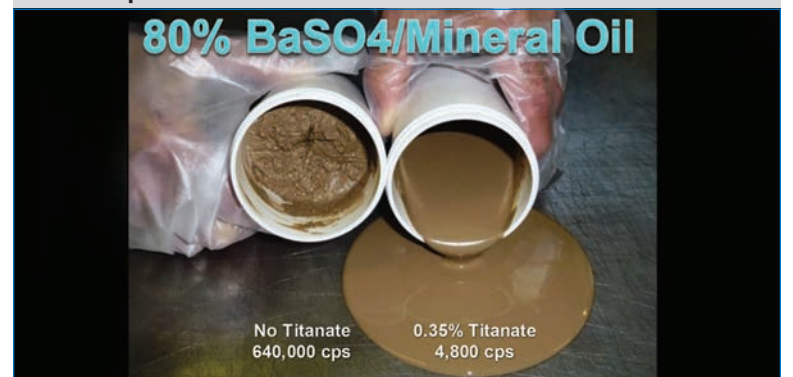
Fig. 6B: 80-percent, non-silane reactive BaSO 4 in mineral oil without and with 0.35-percent titanate.
