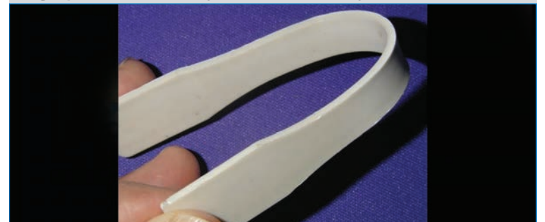
Fig. 6B: 80-percent, non-silane reactive BaSO 4 in mineral oil without and with 0.35-percent titanate.
