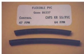
Figure 45 – Extruded flexible PVC (Geon 86337) gray tubing as discussed in Table 38. of 1.0 percent CAPS (KR 55/PVC pellet) permitted a line-speed increase from 46.8 to 63.5 with zone temperatures: 20 to 40 °F lower.
