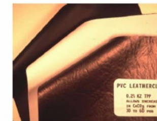
Figure 34 – 0.2% KZ TPP by weight of \text{CaCO}_3 allows increase in filler loading from 30 to 60 phr.
