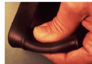
Figure 32 – Flexible PVC washing machine tub splash ring containing 100 parts of \text{CaCO}_3 pretreated with 0.3% KR 44 shows lack of white stress cracking when subjected to 180° bend.
