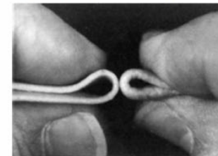
Figure 33 – Both azodicarbonamide foamed PVC plastisol luggage covering samples represent a successful reduction in the PVC: \text{CaCO}_3 ratio from 8:1 to 2:1 (increase in \text{CaCO}_3 from 12.5 to 33.3%) while maintaining excellent film strength using KR 138S. The sample on the left exhibited a reduction in “hand” or feel caused by a tighter cell structure induced by the titanate. The problem was resolved by quick quenching the titanate containing film (left) at 260°C as compared to 210°C (right). Film integrity was maintained and sponginess and the hand of the highly filled composite was better than the (lesser loaded) prior art control.
