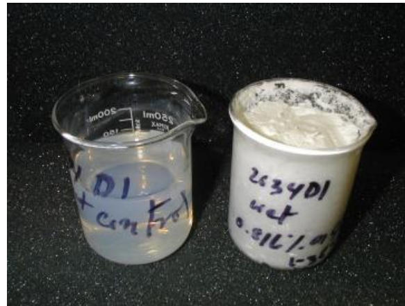
Figure 4 – (Left)-34% 20-nanometer silica sol gel (Nyacol) control with no titanate. (Right)-2.4% LICA 38J exfoliates silica and absorbs the water to form a powder.
