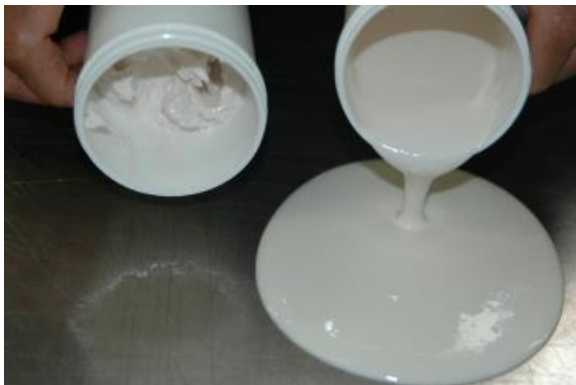
Figure 7 – 60% ATH (Polyfill 402)/40% Mineral Oil – (left) No Titanate – 800,000 cps, (right) 0.7% LICA 38 Titanate added in situ – 9,600 cps.
