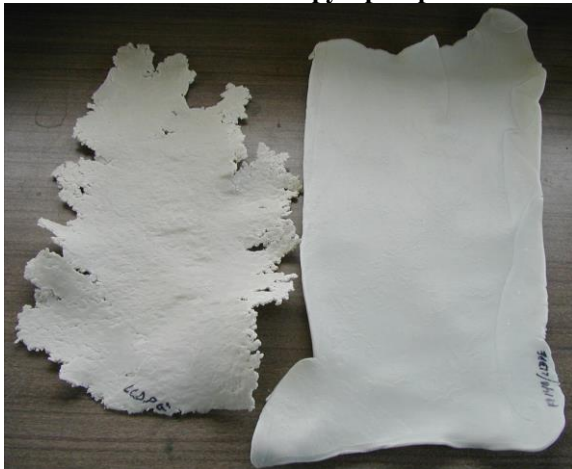
Figure 6 - (Left) 60% Mg(OH) 2 /LLDPE. (Right) 0.7% LICA 38 treated 60% Mg(OH) 2 /LLDPE.
