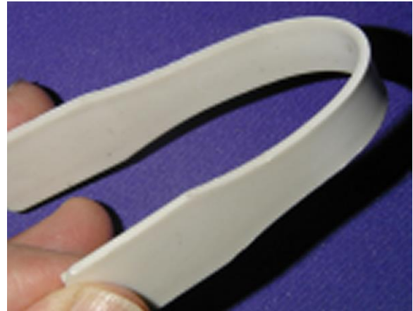
Figure 8 – 70% 3 \mu CaCO 3 filled Polypropylene homopolymer, wherein 0.5% KR TTS titanate treatment by weight of CaCO 3 allows 180° bend of tensile bar with no white stress cracking.
