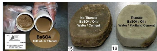
Figure 6: (Left) non-silane reactive BaSO 4 dispersed in mineral oil without & with 0.35% titanate. Function 1 Coupling achieved in situ absent silane hydrolysis. (Right) Oil-soaked spent drilling mud (BaSO 4 ) compatibilized in a water-Portland cement mixture using subject titanates.
