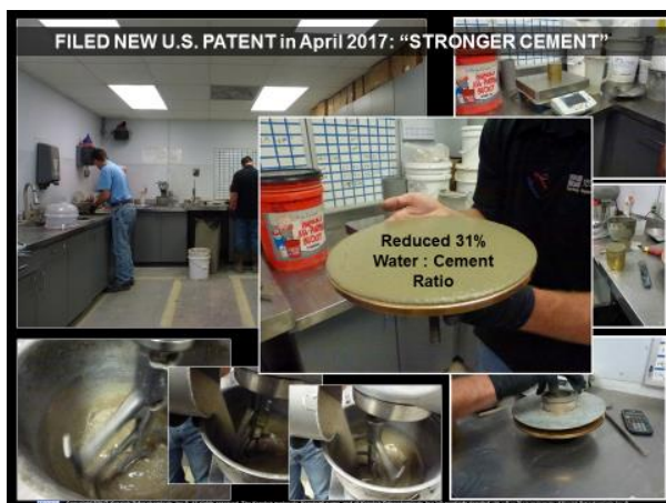
Figure 7: A New 1.5-Nanometer Titanium Treated Portland cement (ASTM C150 – Type I) reduces the cement water ratio by 31% to equivalent slump (flow). Tests conducted at TEC Services Laboratory.
